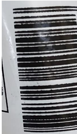
8.2. Poor print quality barcode - not enough contrast between white and black lines
